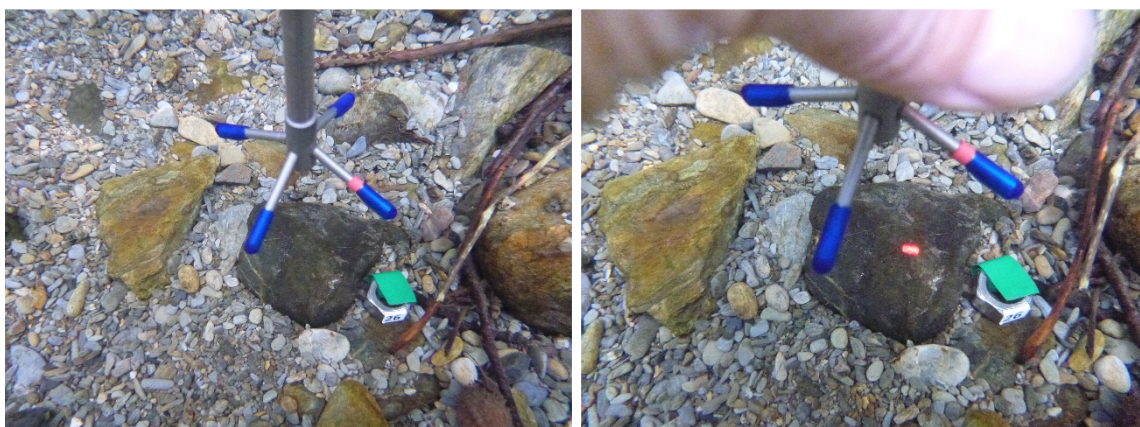
Figure 4. Underwater photos of the sampling location marked with a metal nut (left) and a laser pointer at the precise sampling spot (right).
