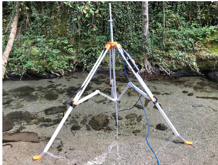
Figure 3. Tripod with attached Vectrino Profiler (Nortek AS, Norway) measuring high-frequency flow velocity at 2 cm above the stream bed.
