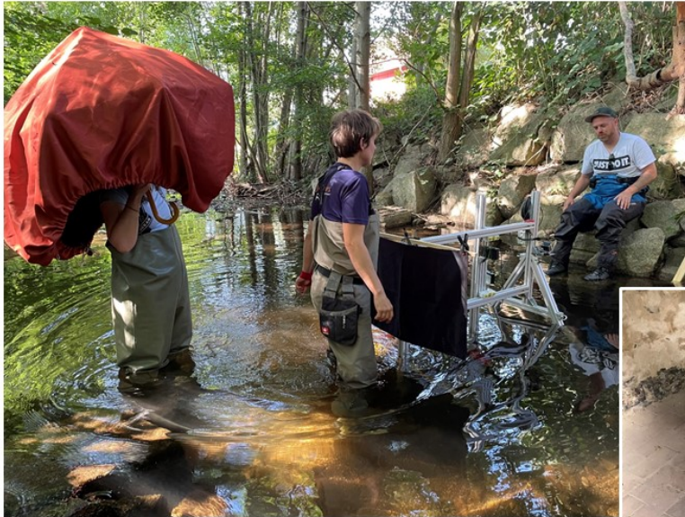
Carboy of tracer addition is also used for calibration of the laser scan
