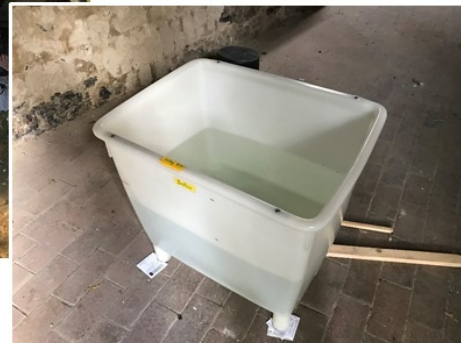
Carboy of tracer addition is also used for calibration of the laser scan
